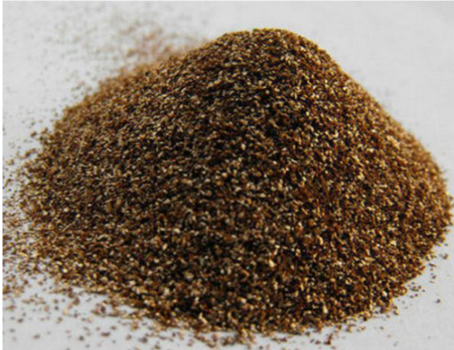
Figure B.1 – Not OK (NOK) – loose absorption material
